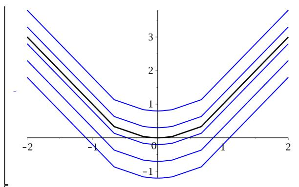
The plot above suggests that all trajectories are parallel to the set S, and terminate at the vertical axis, but only those points starting on the set S (in black) end up at the origin.
