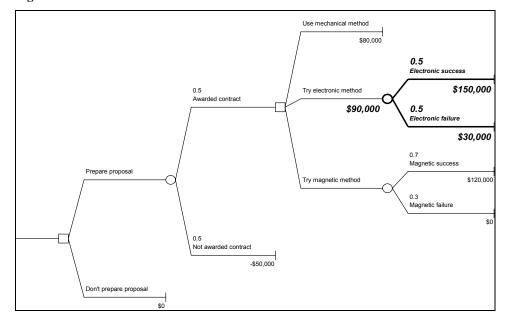
Figure 14.8 Electronic Event Node Rollback Value
