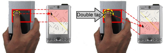
Figure 10. Left: The highlighted input region is mapped to the upper portion of the screen; Right: Double tapping toggles the mapping.
