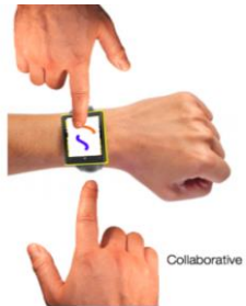
Figure 2. The HWD camera can sense the direction of finger landing on the smartwatch for multi-user sensing.
