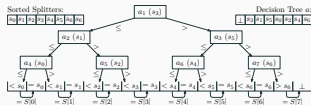
Figure 2: IPS 4 o organizes the pivots in a decision tree structure for quickly finding the correct bucket for an element. Reprinted from Axtmann et al., 2022.
