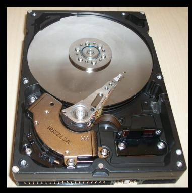
The read/write *head* is on an *arm* that moves to different *tracks* on the *platter*.
