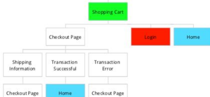
Image 1: Shopping cart branch of site map. It is a direct branch from Home.
